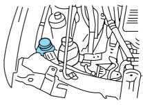
When the engine is cold, check the level of the engine coolant in the reservoir.
